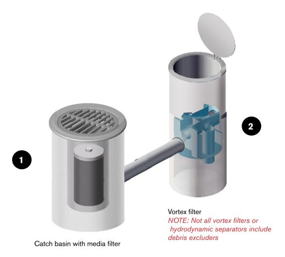
Connections to catch basins and vortex filters shall be through manufacturers' supplied and approved connections or shall be installed with watertight rings or grommets conforming to ASTM C 923 for concrete structures. Field applied PVC & CPVC bulkhead fittings shall conform to ASTM 1784. Polypropelene bulkhead fittings shall conform to ASTM D 4101.
