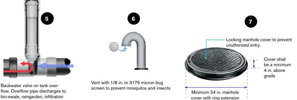
flow. Overflow pipe discharges to bio-swale, raingarden, infiltration device or other approved location. All exposed openings shall be screened with 1/8 in. screen mesh.
