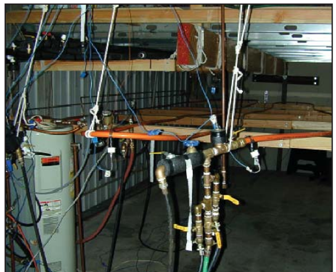
Figure 4. Test Rig for Uninsulated PEX-Al-PEX
