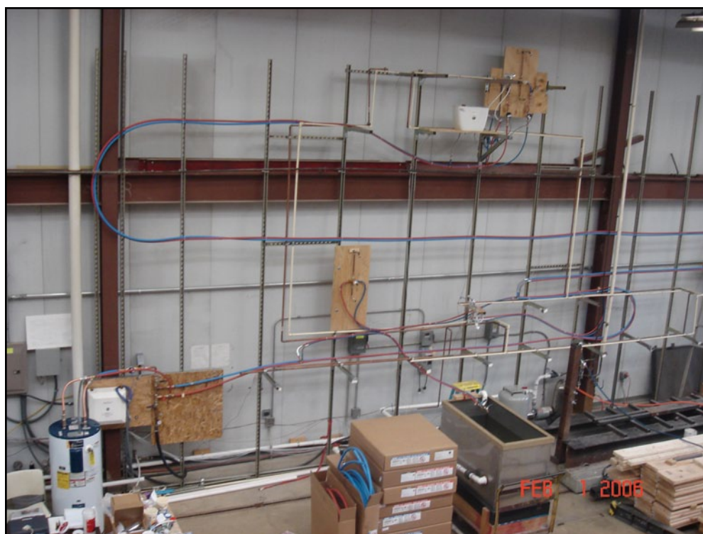
Figure 8.2 – Laboratory Test Set-up with Five Outlets, Hot Water Tank, and T&B System
