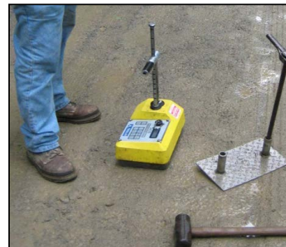
Figure 4: A Nuclear Density Meter calculates density and moisture.
