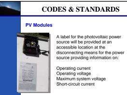
The rated capacity of the module is provided on the back of each panel
