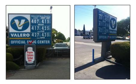
Oops... the building department missed this one. This before and after view shows an encroachment hazard along a path of travel with bottom edge of sign 40 inches above pavement. The sign was <u>not</u> lowered to less than 27 inches above pavement to comply with 2013 CBC Section 11B-307.2, instead a bollard was installed at the end of the sign and 8 inch height grouted masonry curb was installed below the sign to create detection for an individual using a cane.
