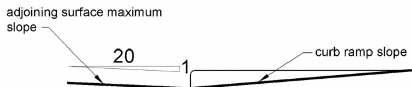
Figure 11B-406.5.7 Counter Slope of Surfaces Adjacent to Curb Ramps
