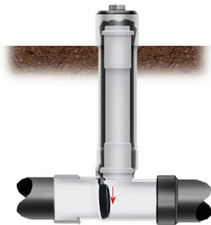
No water in building sewer, flap opens by gravity, rests against ledge
