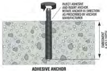
Figure 110: Adhesive anchor installation.
