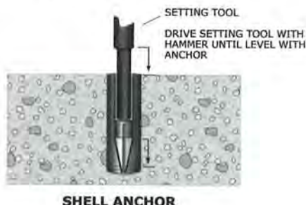
Figure 111: Set shell anchors.
