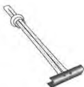
4. TOGGLE BOLT FOR HOLLOW BLOCK FACE MOUNTED
