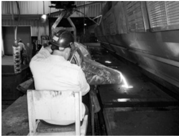
Figure 14—Hand-Pouring of Cast Iron Soil Pipe Fittings.
